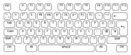
Standard UK keyboard mapping used by the video text overlay unit. By default all UK units are supplied with this.
